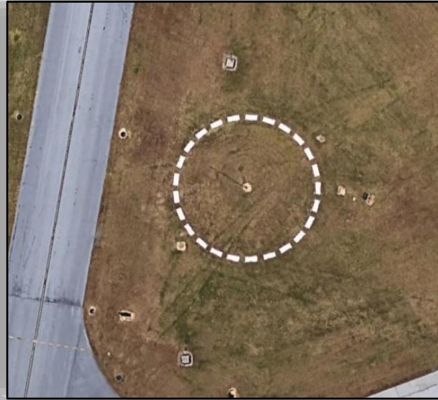
Figure 2-9: Segmented Wind Circle
